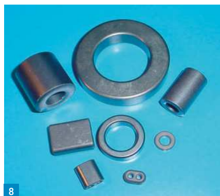
Fig. 1: Circuit to illustrate the operation of a choke. Fig. 2: Signal on channel 1 much larger than on channel 2 (see text). Fig. 3: As (2) but with the choke removed. Fig. 4: Test to illustrate using a choke in a power supply. Fig. 5: Relatively small AC content superimposed on the DC. Fig. 6: The rectified waveform. Fig. 7: Output with the choke disconnected. Fig. 8: All grey (ferrite) cores. Fig. 9: Coloured (iron) dust cores. Fig. 10: Self resonance is due to the inherent capacitance and resistance in any coil.
