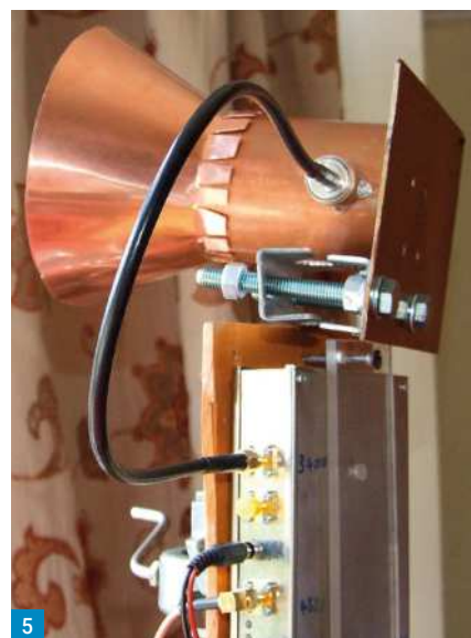
Fig. 1: PCB antennas, top left clockwise: Kent 23cm 2 ele Yagi, Kent 2-11GHz LPA, Kent 2.4GHz 5 element, 3.4GHz 7 ele from SG Labs. Fig. 2: The Bi-Quad and Double Bi-Quad with connection inset. Fig. 3: The basic antenna arrangement. Fig. 4: The 67mm tube with probe fitted. Fig. 5: The finished 3.4GHz antenna with flare on SG Labs transverter. Fig. 6: My 10GHz horn and feed arrangement. Fig. 7: The 60cm dish and feed arrangement.
