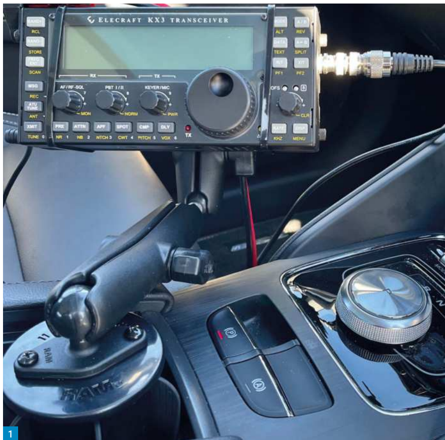
Fig. 1: The RAM mount for the KX3. Fig. 2: The AX1 gutter mount.
